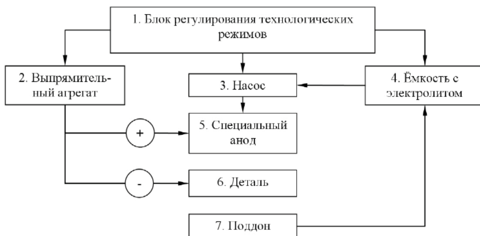
Рис. 2. Схема установки нанесения гальванопокрытий методом натирания. Fig. 2. Flow-sheet of local plating device. 1. – controlling block for the adjustment and maintaining process parameters; 2. – rectifier; 3. – pump; 4. – container with plating solution; 5. – special anode; 6. – plated object; 7. – anti-spilling dish
