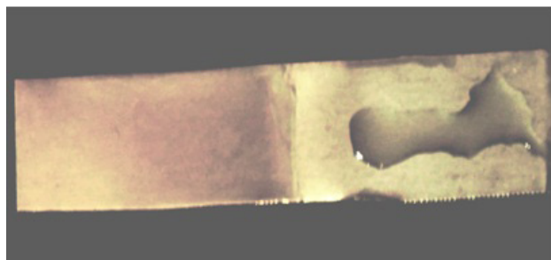
Рис. 2. Общий вид образца, наполовину обработанного в растворе ЦКН-60Ti Fig.2. General view of treated (left) and non-treated (right) surface of titanium
